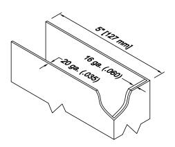
20 ga. Channel (.035) + 16 ga. (.060) Support Strip adds an additionnal (.095) or 3/32" (2.4 mm) to the edge of your door. When sizing your door for the opening you must allow 3/32" (2.4 mm) on each leaf.
