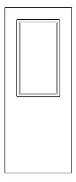
Low Profile Beveled VISION LITE with continuous glass retainer. Recommended for applications where low profile, total visibility and light transmissions are required.
